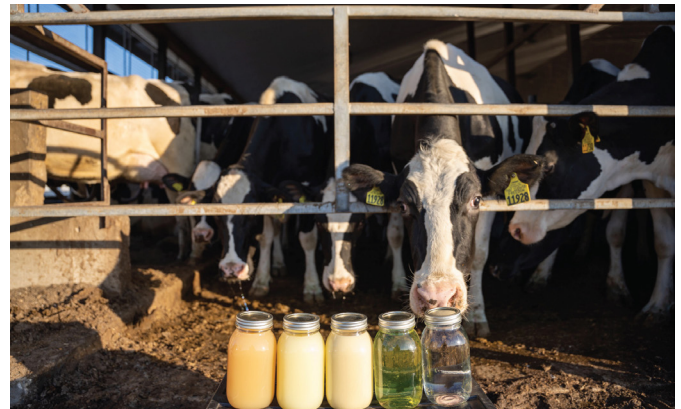
Figure 2: (left to right) Raw WW batch 1, raw WW batch 2, ZwitterCo SF Concentrate, ZwitterCo SF Permeate, RO Permeate.
